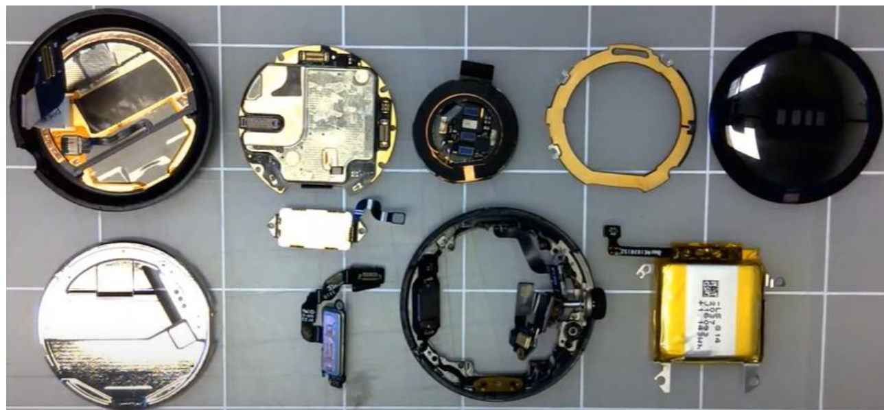
图：Google Pixel Watch拆解
